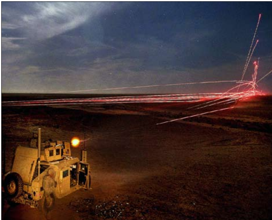
Below: Tracers from a machine gun illustrate the characteristics of danger space and beaten zone over ground. Good gunnery means learning how to establish and control this "fence" of coordinated fires.
